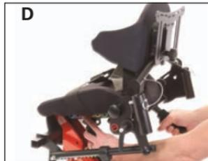
**To adjust to a longer seat depth setting,** adjust the seat tube (seat depth) first by depressing the spring button and moving only one hole at a time. Then adjust the following arm (back angle) no more than two holes at a time. Continue this sequence until you achieve the desired setting, and the colors on the seat tube and following arm match (C).
